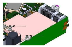
• Place thermal pad to the heat sink plate.
