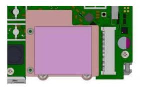
• Install module to the miniPCIe slot and secure with previously removed screws. Tightening torque 0,3 Nm.
