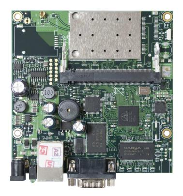
The RB411AR is has a built-in 802.11 b/g wireless card with a sturdy MMCX connector, and a spare miniPCI slot for another wireless card.
