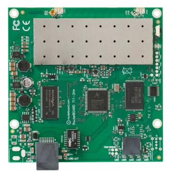
The RB711 is a small CPE type RouterBOARD wireless router with an integrated 2GHz 802.11b/g/n wireless card.
