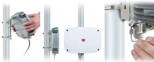
Corrosion resistance is enhanced by using only high grade materials. Enclosure is made of diecasted aluminium and covered with UV resistant coating. All hardware is made of Stainless Steel. Body screws are captive, they do not fall out when released.
