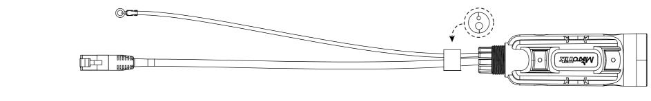
2. Take the rubber plug and fit it onto the cables. The cables must be placed in the matching hole size of the rubber plug. Push the rubber plug into the Outdoor case.
