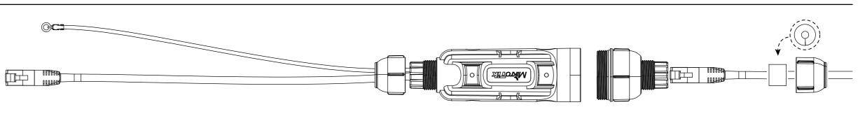
3. Follow the diagram sequence for inserting your ethernet cable. Lastly screw the Small Caps on both ends onto the Outdoor case tightly.
