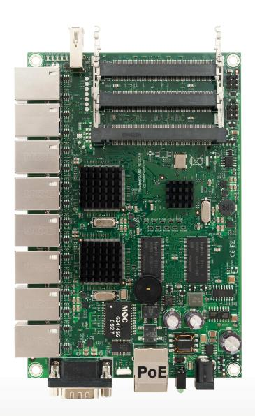
The RB493G has nine Gigabit ethernet ports, three miniPCI slots, and a switch chip, so the ethernet ports 2-9 can be grouped together to make it act as a switch.
